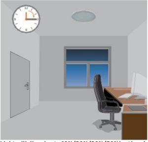
Light will dimming to 10%/20%/30%/50%(optional via set key) after the hold time when no object movement within detection ranges.
